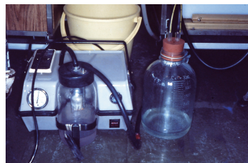
Figure 3 'Dry dialysis'. Water was removed by a negative pressure pump (left in the picture)
